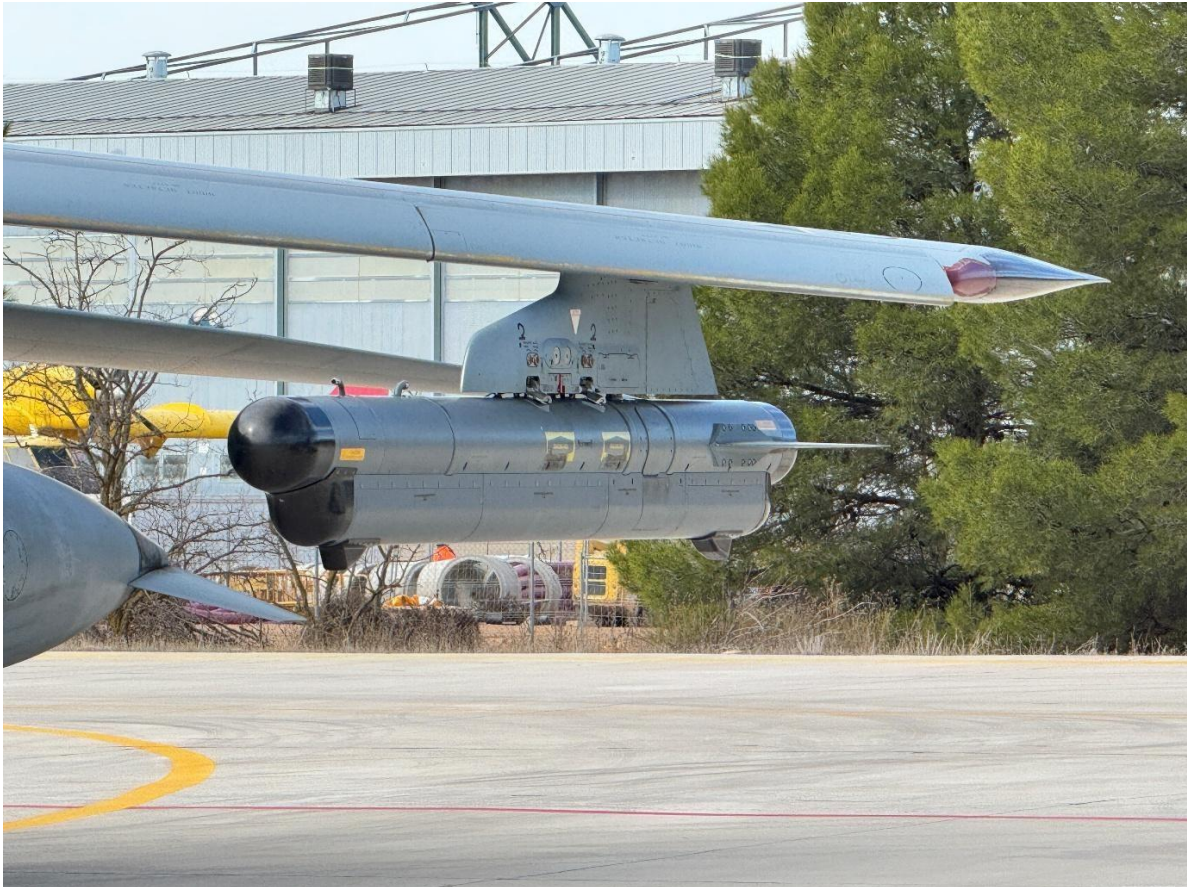
Cerberus ECM pod, "Tornado Self-Protection Jammer" (TSPJ). Foto: autor .
